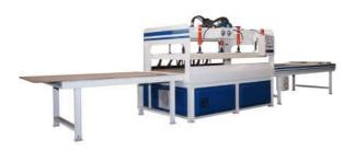
This machine uses high frequency to dry wood glue fast. Usually used in the laminating process or press veneer for doors. This machine can drying glue in just two minutes without causing any changes to structure of the material. Suitable for those who pursuit of speed and quantity. This machine is better than Hot Press. Hot Press can only cover one side, with HF Laminating you can dry multiple sides at once without having to flip the material and dry within 5 minutes.
