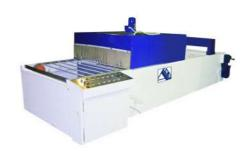
Heat Shrink or Shrinking Packing allows wrapping the product by tightening the plastic wrap around the product by heating it in a machine. So that the product is safe from the presence of water and dust. This machine has automatic temperature control that you can adjust according to the heat needed.
